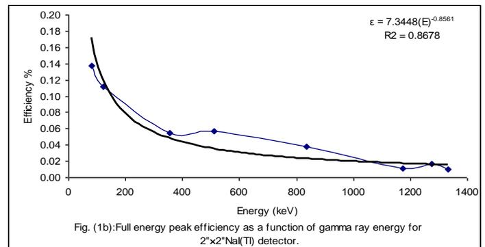
Fig. (1b):Full energy peak efficiency as a function of gamma ray energy for 2"×2"NaI(Tl) detector.
