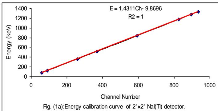
Fig. (1a):Energy calibration curve of 2"×2" NaI(Tl) detector.
