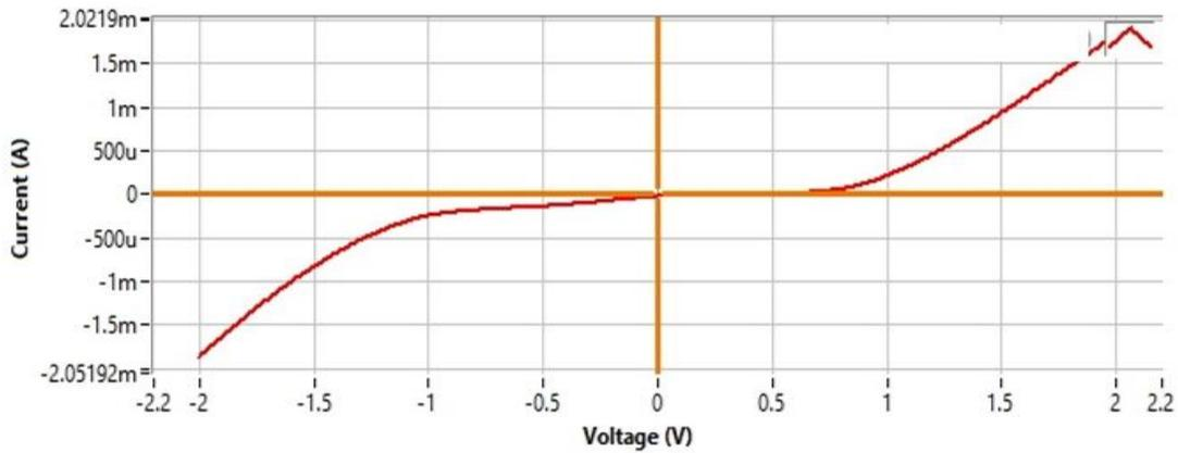
**Figure 3 (a):** I-V characterization of the solar cell with 5% pomegranate dye solution
