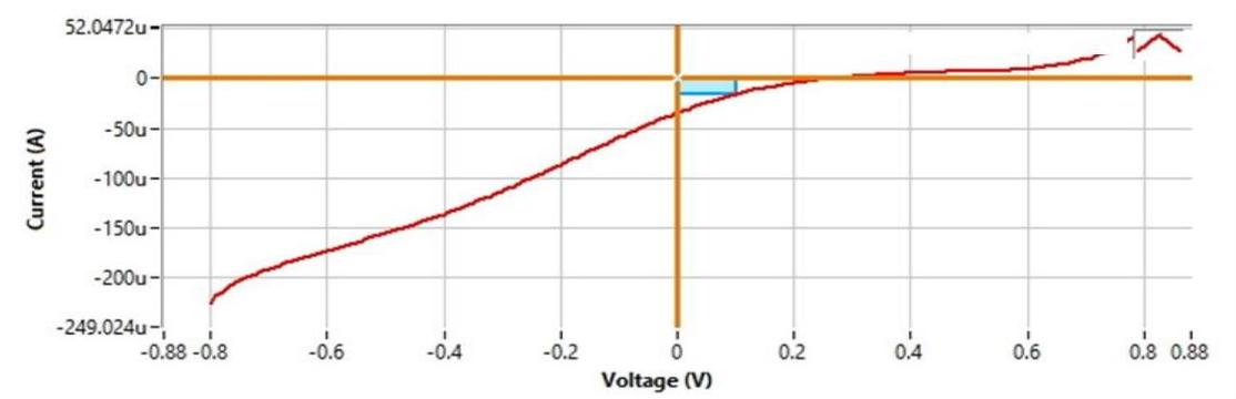
**Figure 3 (b):** I-V characterization of the solar cell with 10% pomegranate dye solution
