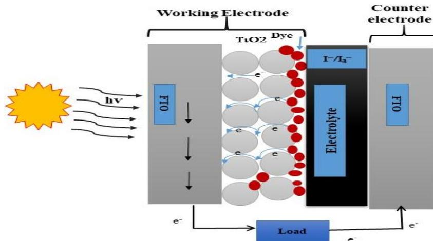
**Figure 1:** The pictorial representation of the working mechanism of DSSC
