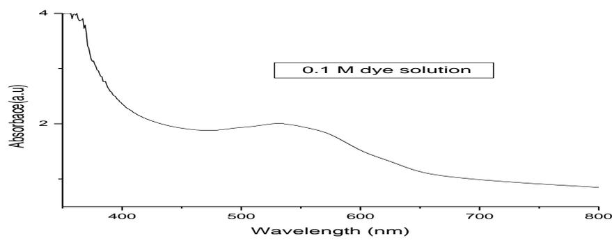
**Figure 2 (a):** The UV-Vis absorbance of 5% concentration of pomegranate dye
