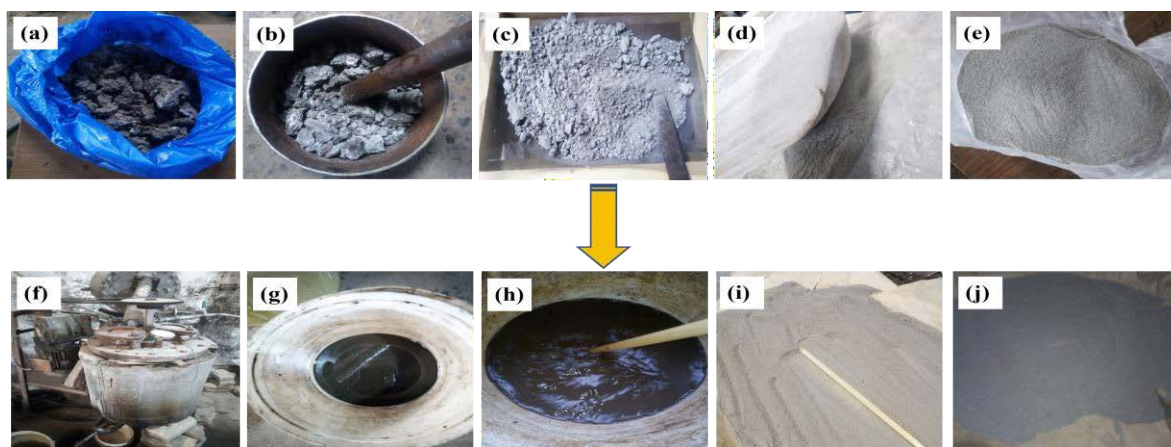
Figure 4. Grinding (a-e), modification in DMSO and drying of MMT (f-j)
