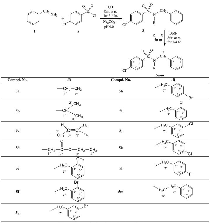
Scheme-1: Synthesis of N-substituted sulfonamides, 5a-m
