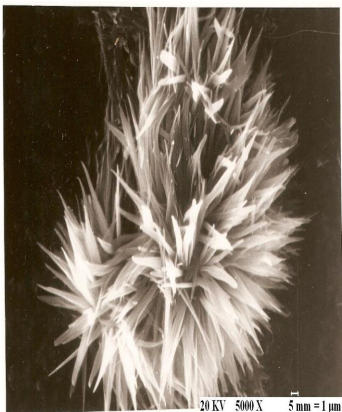
Fig-3(a,b): SEM micrograph of lily-like copper plants grown in polymer template
