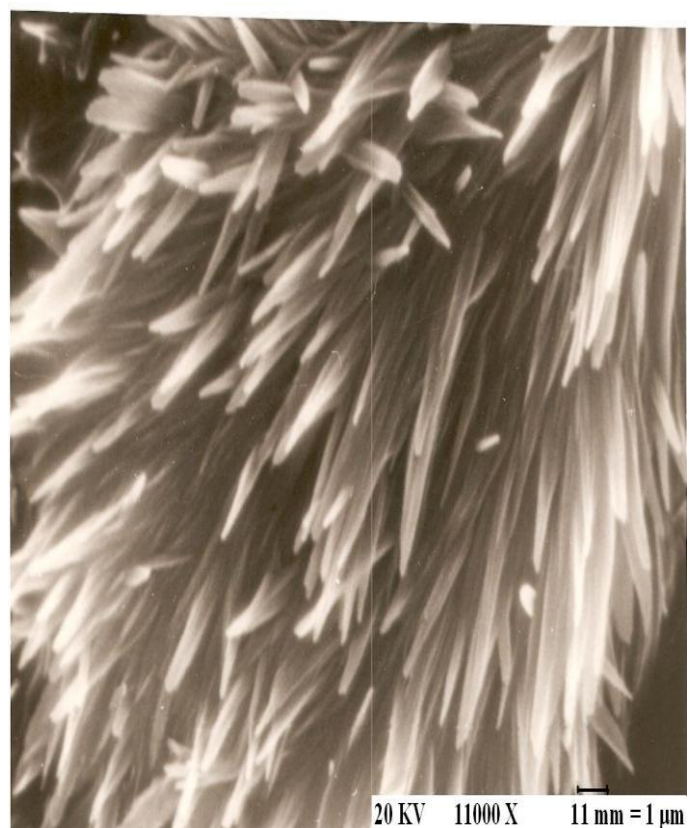
Fig-3(a,b): SEM micrograph of lily-like copper plants grown in polymer template
