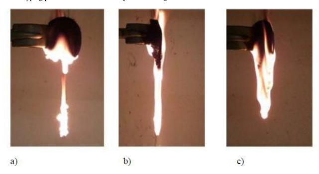
Fig.11: a) Polystyrene b) P.S with alumina c) P.S, Mg (OH) 2 with alumina
