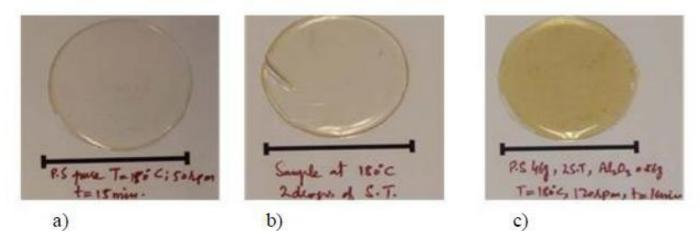
Fig-5: a) Polystyrene b) P.S with S.T c) P.S with S.T and Mg (OH)<sub>2</sub>
