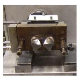
Fig-3: Brabender Plasticorder; (a) Mixer with control panel (b) Mixing screws
