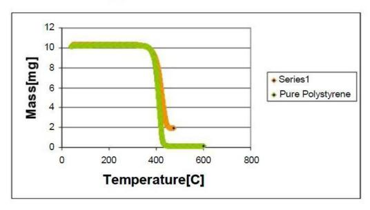
Fig-9: TGA Analysis (Polystyrene and Polystyrene Alumina Nano fiber 2%)
